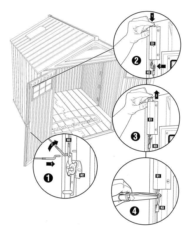
Connect the **BOTTOM CABLE** (**H4**) by inserting the "z-hook" end into the hole at the bottom of the **SWIVEL LATCH** (**H2**) and rotate into position.
